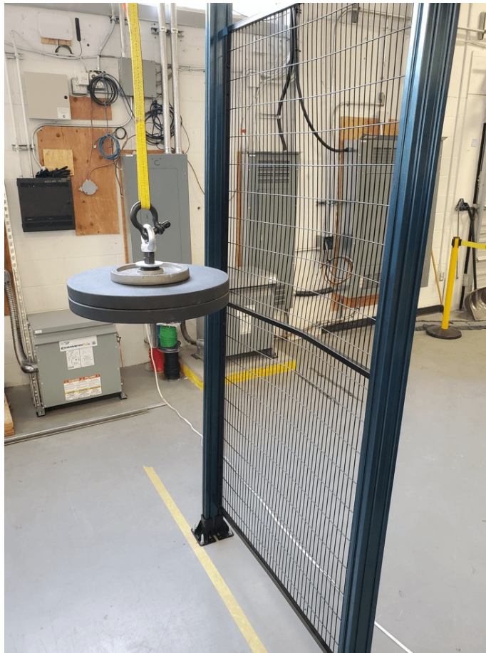
Post-impact deformation of machine guarding panel
