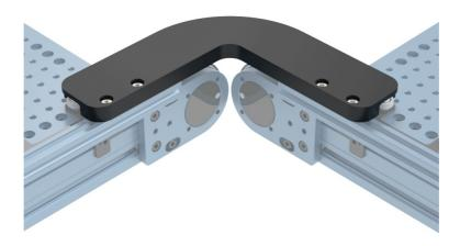
As its name suggests, this HDPE corner guide engages with the bearings of the pallet guides to smoothly change the direction of the pallet. The right-angle guide attaches atop the 22.5mm extrusion through the 4 counterbored holes.
